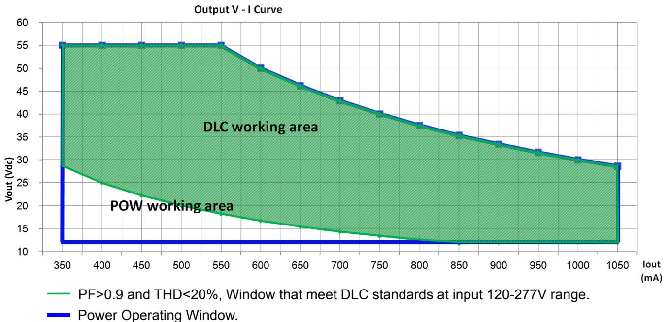
Note: When the output current is set, the output voltage is automatically limited within the curves.
