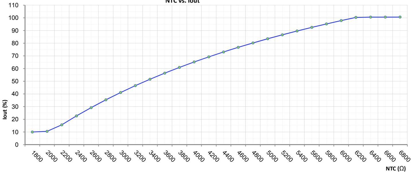
Note: Maximum dimming current is limited by NTC.
